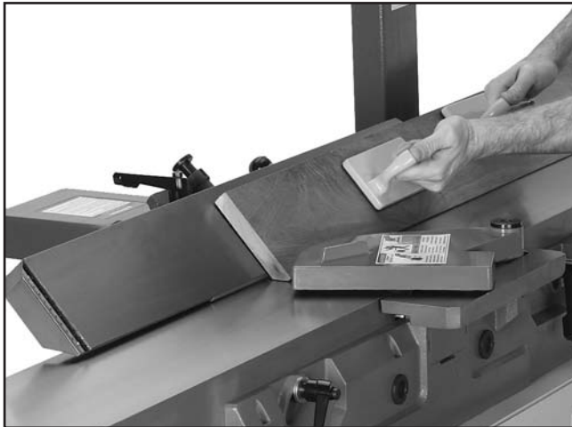
Figure 41. Fence setup for a bevel cut of 45°.
